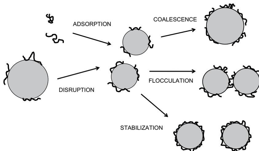
**Fig. 1.** Illustration of main physico-chemical processes involved in making of emulsions. Stabilization of fine droplets requires mechanical disruption of coarse droplets accompanied by rapid effective adsorption of emulsifier at the new oil–water interface. Collision of droplets with insufficient coverage of emulsifier leads to coalescence and/or flocculation.
