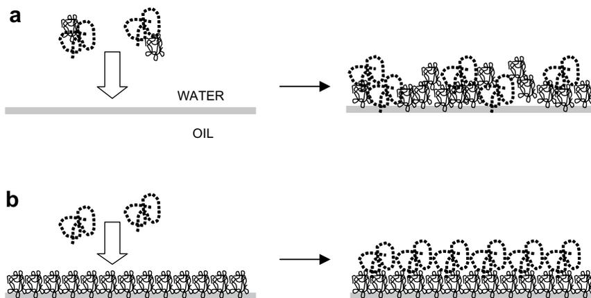
**Fig. 7.** Illustration of two alternative ways of making a composite layer composed of protein-polysaccharide complex at the oil-water interface: (a) the complex previously formed in solution adsorbs at bare interface; (b) the polysaccharide adsorbs onto a previously formed protein monolayer.
