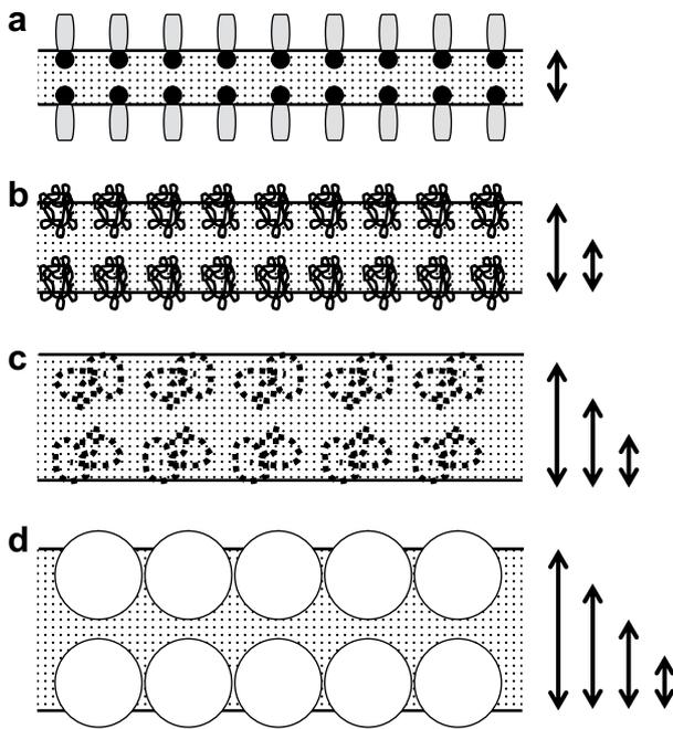
**Fig. 3.** Schematic representation of relative thicknesses of thin films between closely approaching oil droplets stabilized by (a) surfactants, (b) proteins, (c) hydrocolloids and (d) colloidal particles. The diagrams illustrate effects of differences in sizes of the different kinds of adsorbed species, i.e., surfactant molecules (0.5–1 nm), proteins (1–5 nm), hydrocolloids (5–10 nm), and particles (10 nm to several  $\mu\text{m}$ ).
