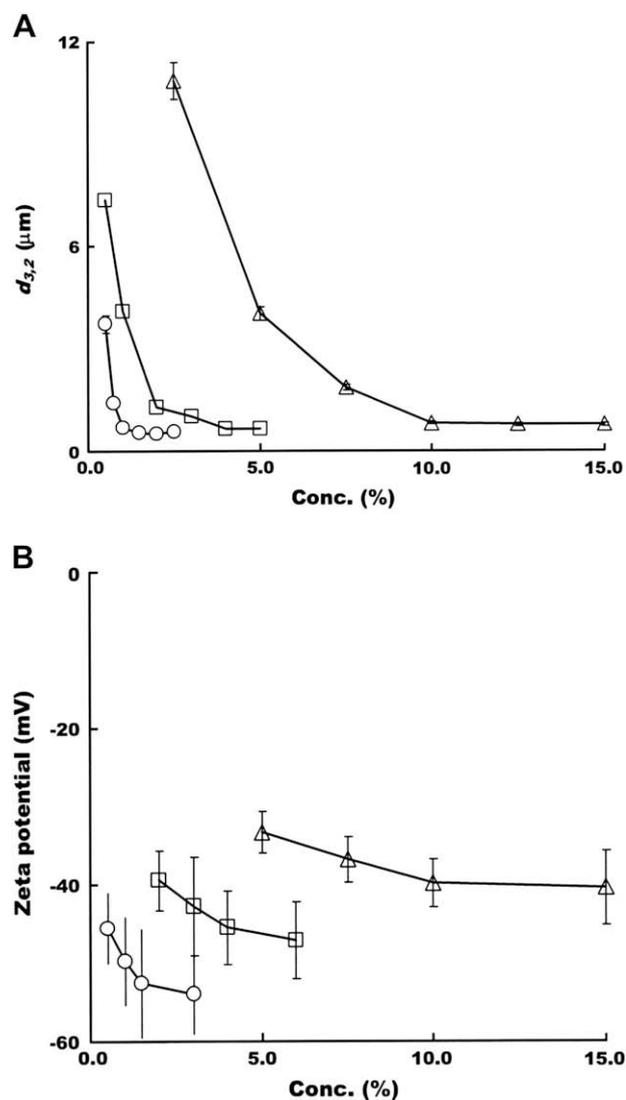
Fig. 2. Comparison of properties of freshly made emulsions (15 wt% triglyceride oil, pH = 3.0) prepared under controlled hydrodynamic conditions with three different food hydrocolloids:  $\Delta$ , gum arabic;  $\square$ , soybean soluble polysaccharide;  $\circ$ , sugar beet pectin. Plotted against the hydrocolloid emulsifier concentration are (A) mean droplet diameter  $d_{3,2}$  and (B) zeta potential. (With permission from Nakauma et al., 2008.)
